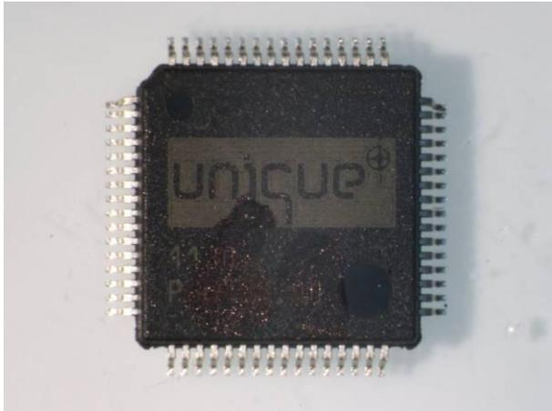
Figure 37: Package after front side decapsulation. (No more Cu wires)
